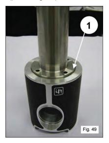
Place the stem in a vice, closing the teeth of the vice on the two flat areas, and proceed with setting, using a torque wrench (pos. 1, fig. 50) as shown in section 3, "Screw tightening settings".
