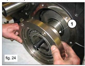
Lay the crankshaft on the bottom of the crankcase. Separate the bearing support cover from the bearing, using a striking hammer (pos. 1, fig. 25).
